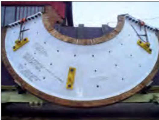
Ball Mill head in halves
