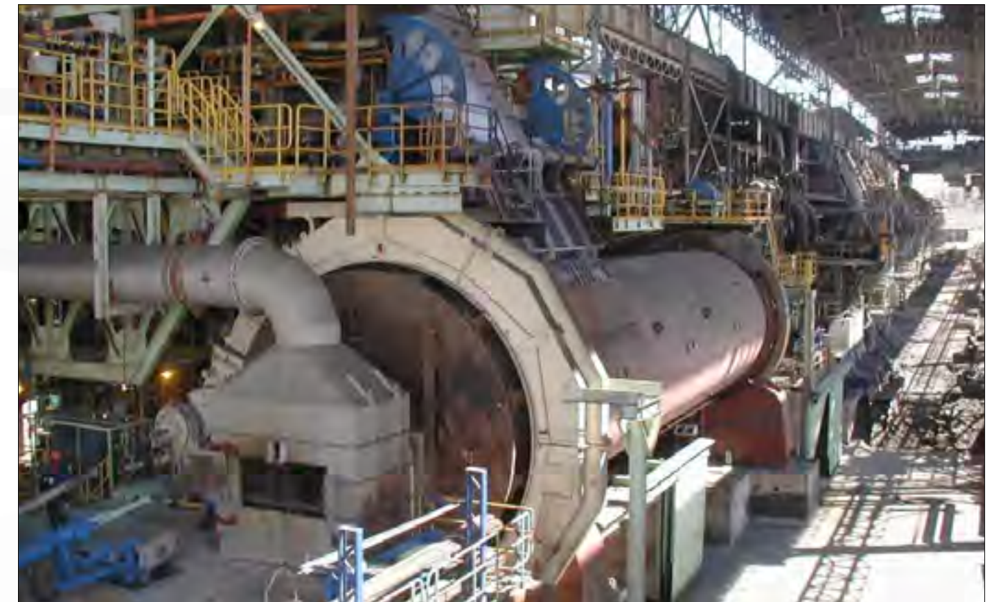
Support rings (cast steel or ductile iron)
