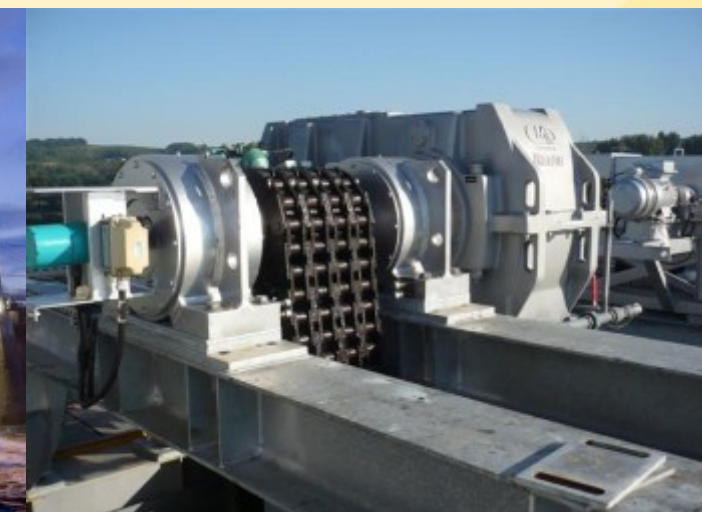
Twin side gearboxes - central drive - couplings - motors - chains - monitoring for 8 doors
