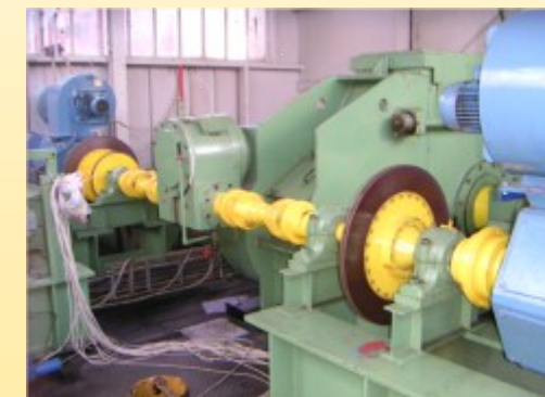
Bogiflex - gear coupling
